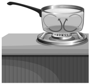
You can see these currents when you boil rice in water. Convection currents also allow heated air to circulate through a room.
