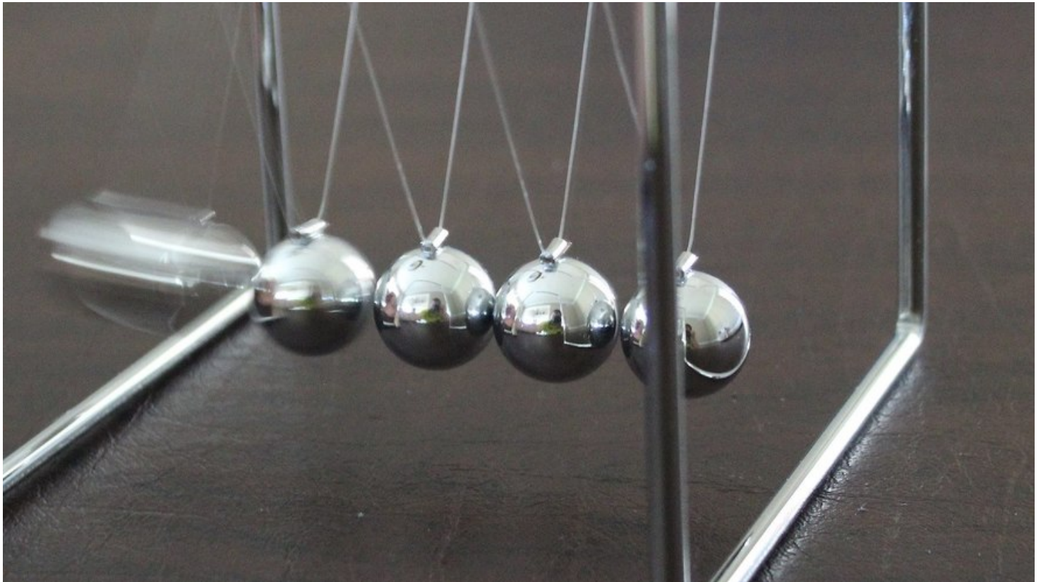
Image 1. Newton's cradle is a device that demonstrates the transfer of kinetic energy. Photo from: Wikimedia Commons
